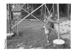
Although disc brakes may seem like a good idea, they are not fail-safe. If the cable breaks in violent storm, for example, an operator would be helpless to stop the turbine. There's no way to apply the brakes!
