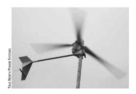
to rotate the machine around the yaw axis. However, the tail resists this rotation and keeps the rotor facing into the wind.
