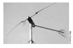
Fig. 5.6: Side Furling. This wind turbine is not broken, it is side furling in high winds, which slows the rotor and protects the machine from damage.
