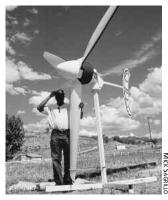
Fig. 3.1a and 3.1b: Wind Turbine Design. (a) The generators in many small wind turbines are housed in a protective case made from aluminum or fiberglass. (b) Others, like this one, are not.
