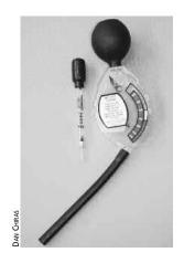
a measure of the density of battery acid. Density is related to the concentration of battery acid — the higher the concentration, the higher the specific gravity. If significant differences in the specific gravity of the battery acid are detected in the cells of a battery bank, it is time to equalize.
